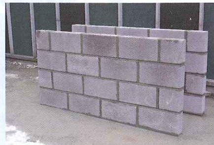
Concrete blocks using University of Glamorgan's cement derived from recycled wastepaper ash
